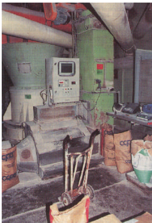
Adding micro-ingredients at a hand tip point is probably the most common practice
